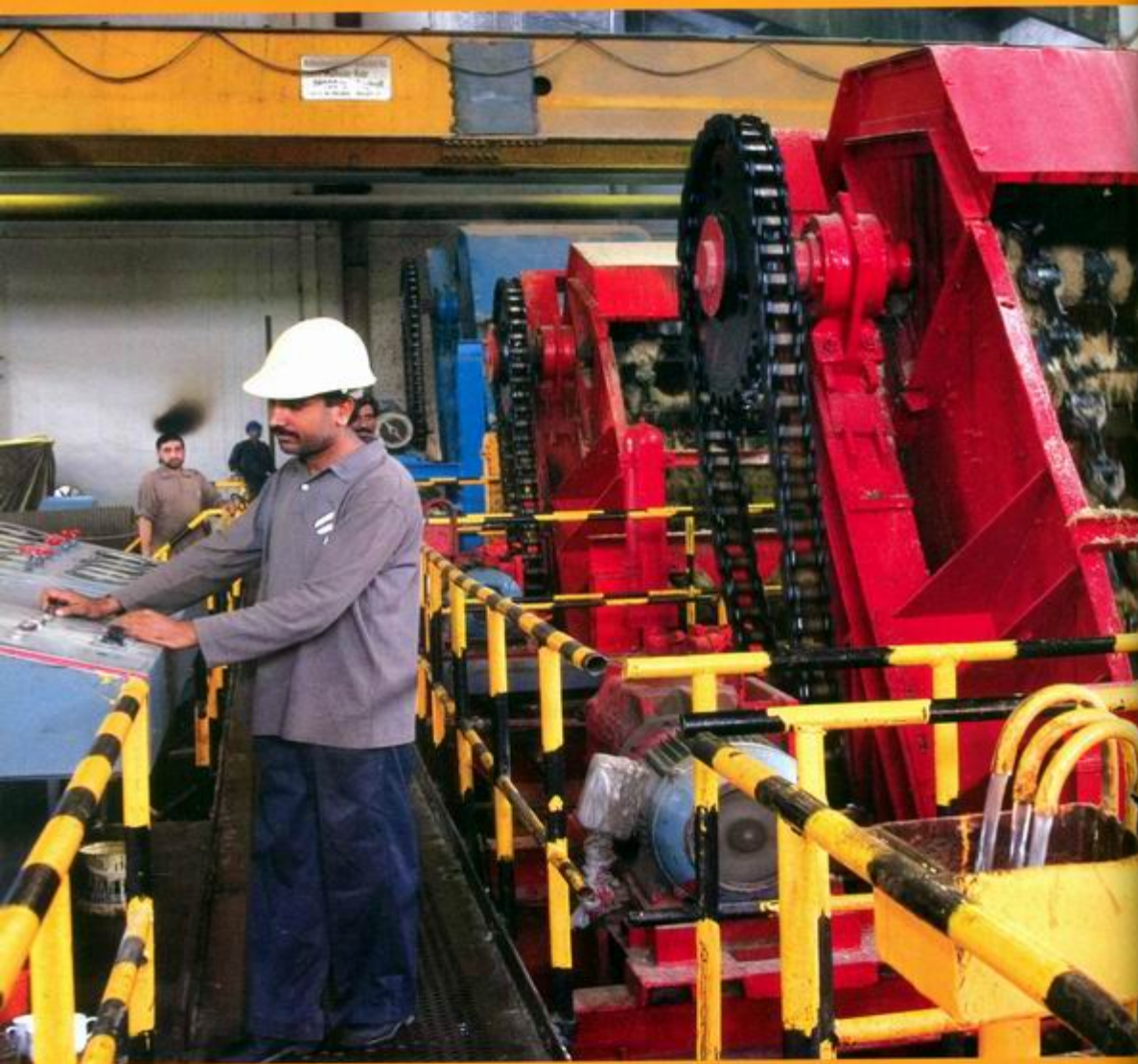
The Mill House, where juice from the sugarcane is extracted on these large machines initiating the sugar-making processes.
